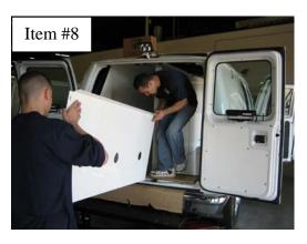
Place **Passenger-side Ceiling** section into vehicle
